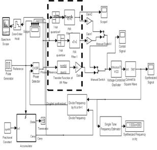
Fig. 2. PLL Frequency Synthesizer Simulation Model
