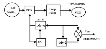
Fig. 2. Fractional-N PLL block diagram
